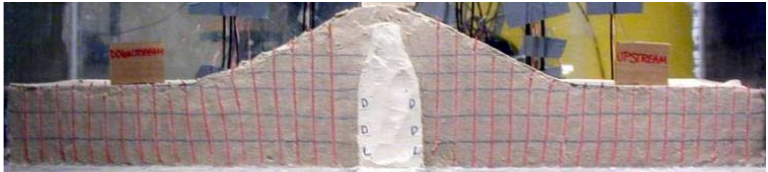
Varying thickness of liquefiable layer
